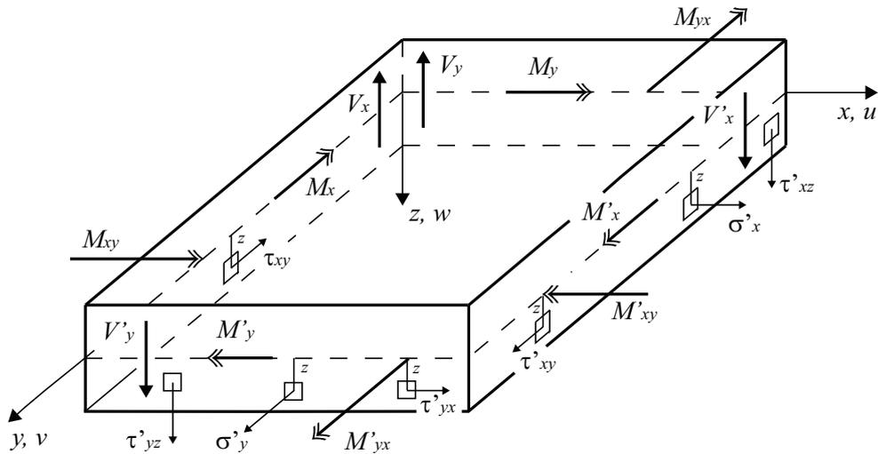
Figure 5: Equilibrium of a rectangular plate element.
