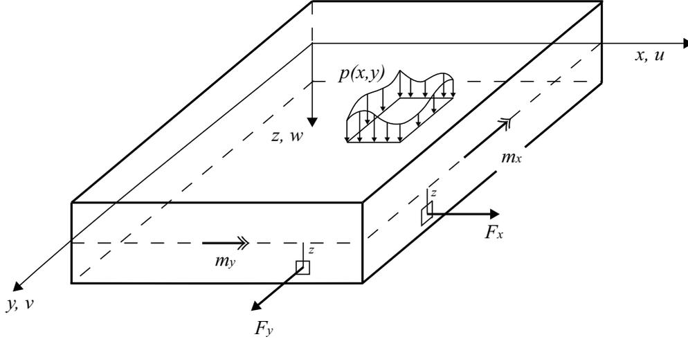
Figure 4: Generalized loads acting on a rectangular plate element.
