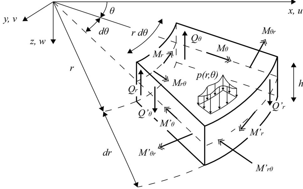
Figure 6: Equilibrium of a circular plate element.
