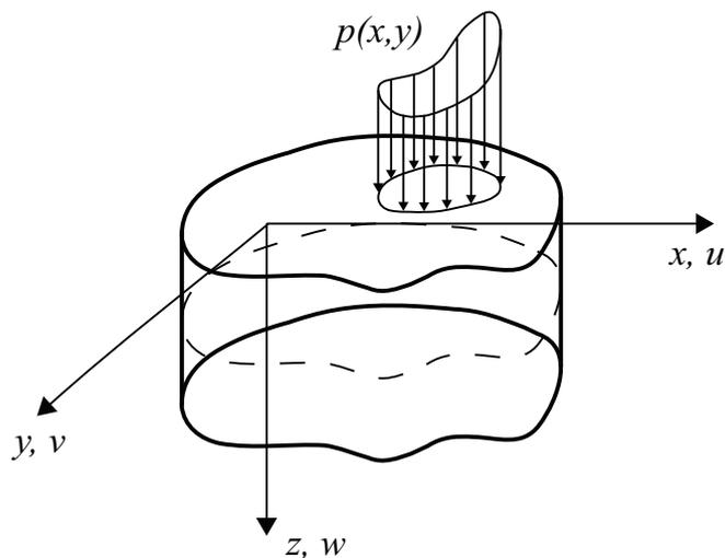
Figure 1: A generic plate element with the reference system lying on its middle plane.
