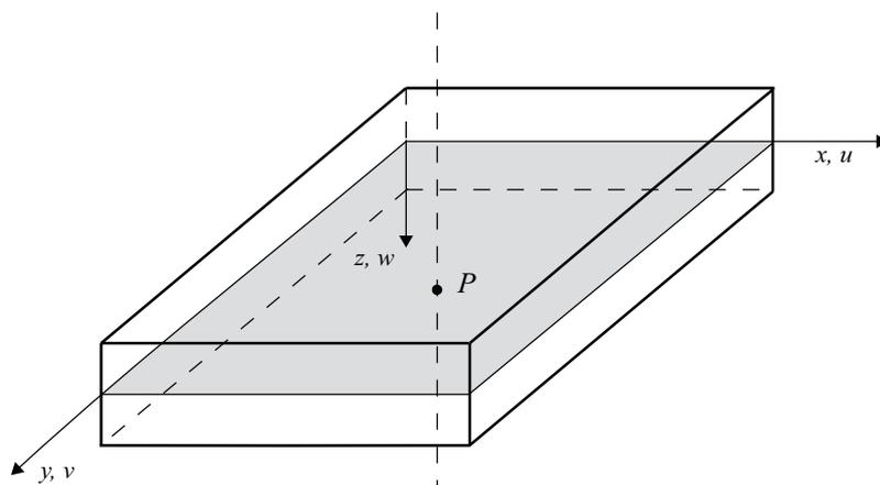
Figure 2: A generic point on the generic straight segment initially orthogonal to the plate middle plane.
